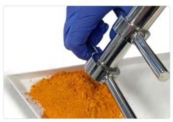
Sample being discharged from a Standard Slot Sampler without a Bottle Holder
