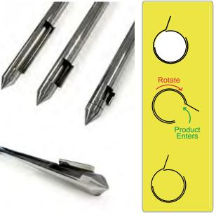
Rotate the whole sampler to take the sample
