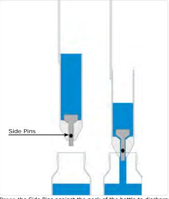
$\mbox{\sc Press}$  the Side Pins against the neck of the bottle to discharge the sample
