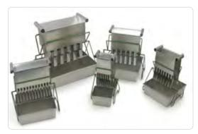
Sample Splitters (Rifflers) are used when dividing and reducing the bulk sample. They are ideal for food, environmental and chemical use.
