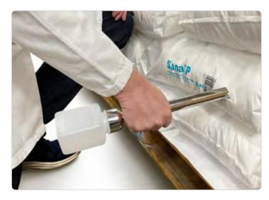
The Sampling Systems Sack Master range has been specially designed to take samples through the side of a sack.
